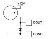
Figure 7 - Digital Output 1 Circuit
